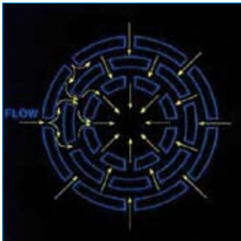
Plan sectional view of a concentric multi cage trim
