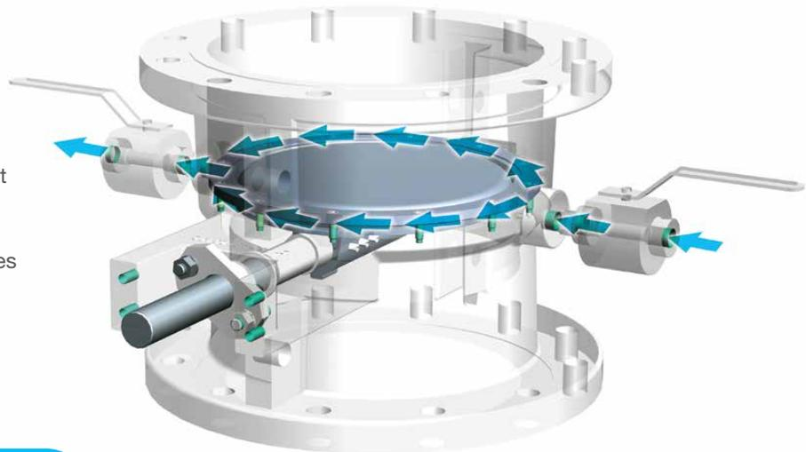
**TYPICAL SEALANT FLOW PATH**
