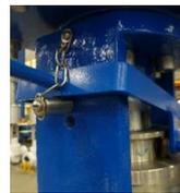
Pin and lever in auto position (Lever Up)
